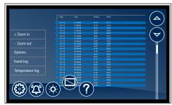
Event Log – to display a chronological listing of events (including errors, Fig. 19 alarms and alerts), touch the **Event Log** label to the left of the screen. Use the UP and DOWN arrows to the right of the screen to scroll through the logged temperatures.
