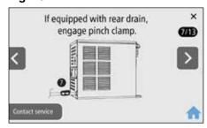
**10.** Hot water tank units: Locate the pinch clamp and engage (close) **(Fig. 26)**.
