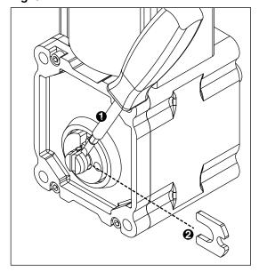
16. Install screw and tighten (Fig. 52.1).
