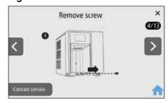
7. Remove the front cover and set aside. Follett recommends setting the cover on the drip tray, which provides a stable base (Fig. 23). Be careful not to stretch or damage any cables connecting the front cover to the unit.
