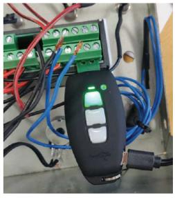
**4.** If the programming fails, the signal leds will turn firmly red instead of green. In this case, repeat the procedure making sure that the programming key is correctly inserted into the controller terminal blocks.
