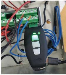
2. If the programming fails, the signal leds will turn firmly red instead of green. In this case, repeat the procedure making sure that the programming key is correctly inserted into the controller terminal blocks.
