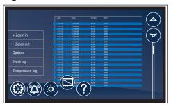
Event Log – to display a chronological listing of events (including errors, Fig. 19 alarms and alerts), touch the **Event Log** label to the left of the screen. Use the UP and DOWN arrows to the right of the screen to scroll through the logged temperatures.
