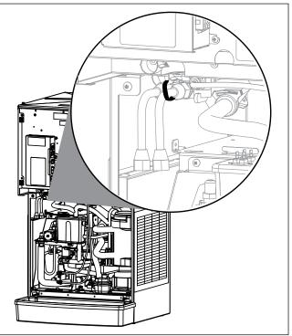
**10.** Lift and position water-cooled lines into hook (Fig. 23).
