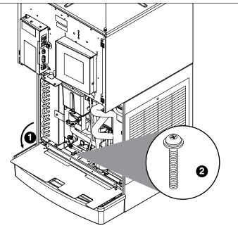
3. Lower drain pan protector (Fig. 20.1). Remove and discard shipping screw (Fig. 20.2).
