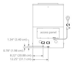
${\bf BS^*}-$  Base stand sold separately; measurements shown are with base stand legs at lowest position. See dispenser detail sheet, form# 6675, for counter cut outs.
