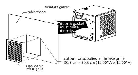
completed installation with gasket and door in place
