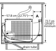
**A:** additional 7.6 cm (3") required if receptacle located directly behind unit.
