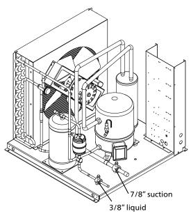
Braze the line set to the suction and liquid lines. Run line set to the docking station and stub in 2".
