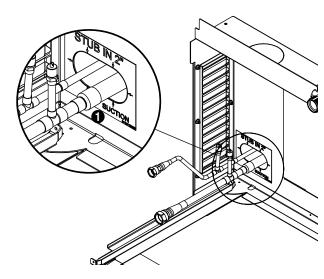
Braze supplied quick-connect lines onto stub-ins ①. DO NOT ATTACH QUICK DISCONNECTS TO EVAPORATOR!
