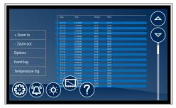
Event Log – to display a chronological listing of events (including errors, alarms and alerts), touch the Event Log label to the left of the screen. Use the UP and DOWN arrows to the right of the screen to scroll through the logged temperatures.
