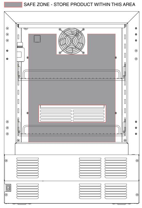
KEEP CLEAR 1" ON EACH SIDE AND TOP. FAN GRILL AND RETURN VENT MUST BE VISIBLE.
