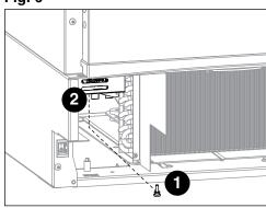
**5.** Pull control module forward 1 inch, rotate left as per **Fig. 7**, and continue to pull the control module forward.
