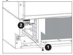
**5.** Pull control module forward 1 inch, rotate left as per **Fig. 8**, and continue to pull the control module forward.
