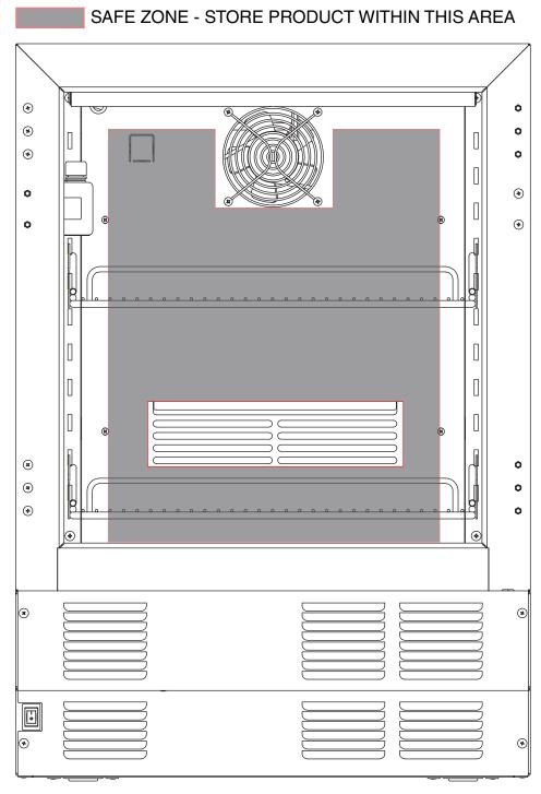
KEEP CLEAR 2" ON EACH SIDE AND TOP. FAN GRILL AND RETURN VENT MUST BE VISIBLE.
