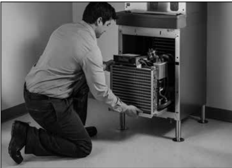
Removable ice machine for easy service
