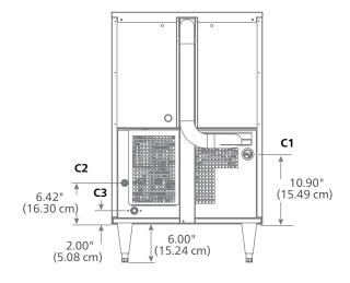
SHORT FORM SPECIFICATION: Ice machine to be Follett model number \_\_\_\_\_\_. Ice machine to be air-cooled and production to be approximately 425 lb (193 kg) per day of \_\_\_\_\_\_ Micro Chewblet or \_\_\_\_\_\_ flake ice at air temp of 70 F (21 C) and water temp of 50 F (10 C). Ice storage capacity of up to 75 lb (34 kg). Ice machine to have stainless steel evaporator, auger, top bearings, heavy duty tapered roller bearings, and low water safety circuit. NSF and ETL listed.
