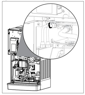
**10.** Lift and position water-cooled lines into hook **(Fig. 16)**.
