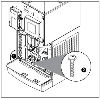
**3.** Lower drain pan protector (**Fig. 13.1**). Remove and discard shipping screw (**Fig. 13.2**).
