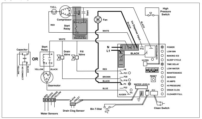
When the dwell time of 20 minutes has expired, the **TIME DELAY** LED goes off. If 5 seconds of ice has been dispensed and the **SLEEP CYCLE** LED (Symphony Plus only) is off, the ice machine will go through the normal start-up sequence when the bin level control signals the control board for ice.
