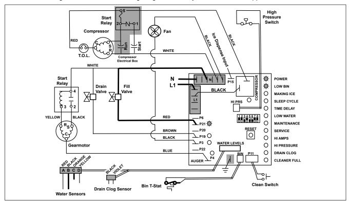
When continuity is seen between B and C, the water valve de-energizes, the AUGER output (P4) comes on along with the **MAKING ICE** LED. The auger gearmotor's start windings are energized through a current style start relay that is pulled in by the initial high current draw of the gearmotor.
