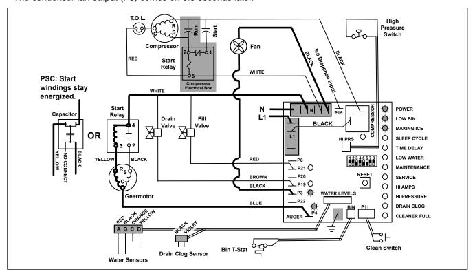
One second (1 s) after the fan comes on, the **COMPRESSOR** output comes on. The compressor circuit uses both run and start capacitors along with a potential start relay. The start capacitor in energized through the normally closed contacts of the start relay.
