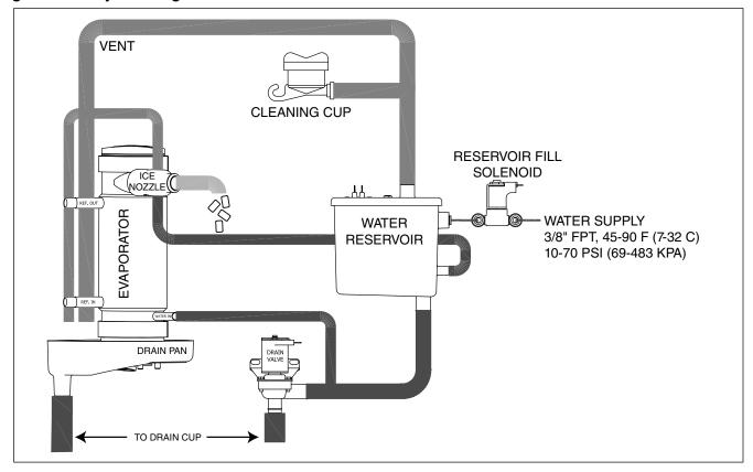
Fig. 7 – Water level diagram
