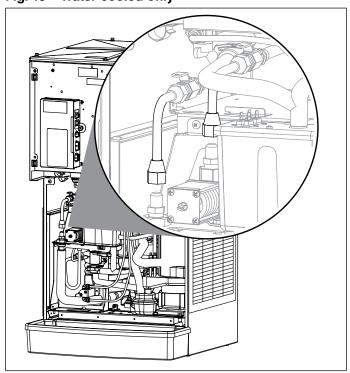
**9.** Shut off inlet and outlet valves to water-cooled condenser and disconnect fittings (Fig. 15).
