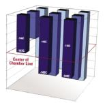
Comparison of temperature distribution in a  $\rm LN_2$  freezer (vapor phase) and Model MDF-C2156VANC-PA | FZRC8-220 mechanically refrigerated cryogenic freezer.
