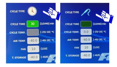
To modify the cycle options, press the tab of the option(s) that need to be adjusted. The tab will light green, you may then adjust the value using the keyboard on the right side of the screen. Once the correct value is set, press the OK button.
