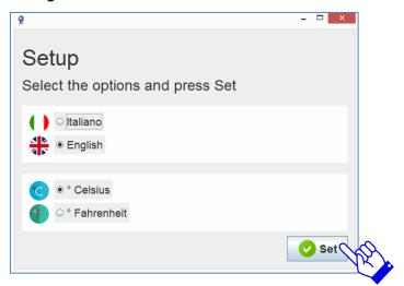
Select the language and scale of temperature, press SET to confirm and exit. Press the Load File tab on the right top of the screen.
