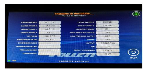
The *Input/Output* menu allows you to check all input signals, such as Temperature Sensors, Door Switch status, and Outputs such as Relays status. (Outputs shown below)
