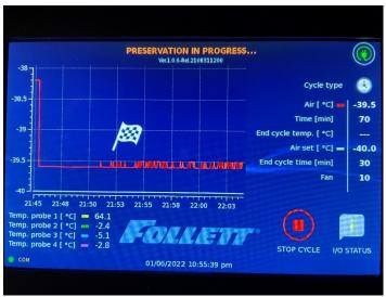
On the right side of the screen, the cabinet temperature, elapsed time from the start of the cycle, end cycle temperature set point, cabinet temperature set point, cycle time set point, and the fan speed are displayed.
