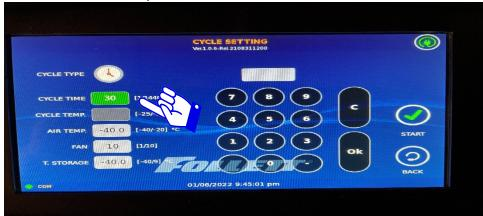
Once the cycle options are set touch the *START* icon to start the cycle: The controller will start to load the program and the following screen will be displayed
