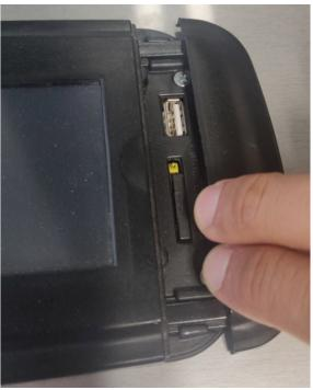
From the USB menu it is possible to upload to the touch screen as well as the PCB software and download the HACCP records.
