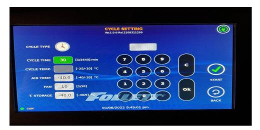
Touch the "CYCLE TYPE" icon to scroll to the desired cycle either by time or by product temperature core probe: For continuous production, use the Time Cycle freezing method identified in (3.1.1).
