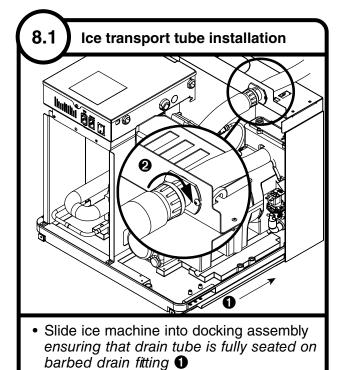
Insert ice transport tube all the way into coupling and tighten nut firmly 2
