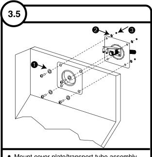
Mount cover plate/transport tube assembly on outside of dispenser using screws, flat washers ①, lock washers ② and nuts provided ③
