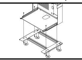
Mount docking assembly to machine stand accessory
