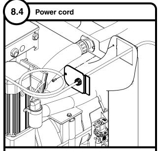
Position plate into opening and secure with supplied screw
