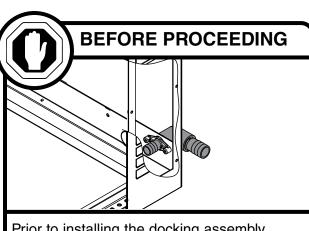
Prior to installing the docking assembly, ensure that the drain fitting is oriented (right or left) correctly for your installation. An optional straight drain fitting is also supplied. You may need to remove the back panel of the docking assembly in order to re-orient or change the drain fitting. Replace back panel prior to mounting the docking assembly.
