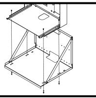
Mount docking assembly to wall bracket accessory
