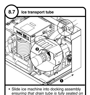
· Insert ice transport tube into coupling and
