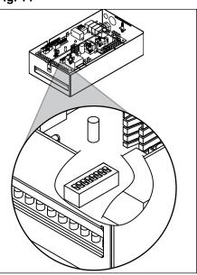
Not used (OFF position) Ice only No internal filter Not used (OFF position) Not used (OFF position) 15 minute delay Not used (OFF position) Six-month PM enabled
