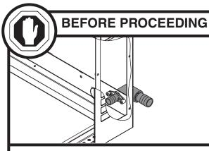
Prior to installing the docking assembly, ensure that the drain fitting is oriented (right or left) correctly for your installation. An optional straight drain fitting is also supplied. You may need to remove the back panel of the docking assembly in order to re-orient or change the drain fitting. Replace back panel prior to mounting the docking assembly.
