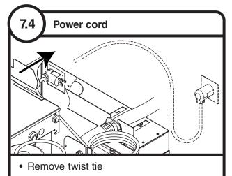
Carefully pass cord thru opening and plug into wall outlet
