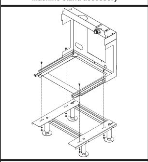
Mount docking assembly to machine stand accessory
