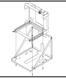
Mount docking assembly to wall bracket accessory
