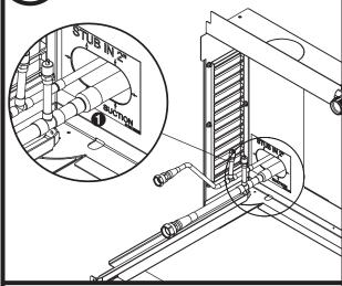
Braze supplied quick-connect lines onto stub-ins 1.
