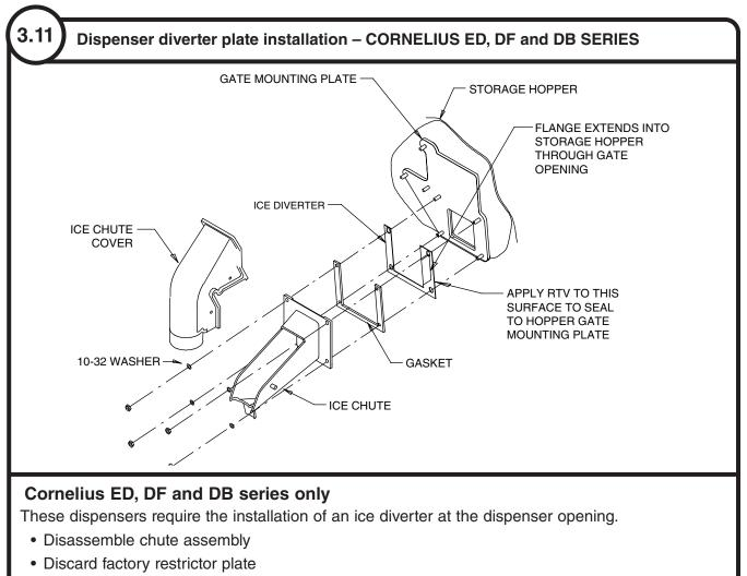
• Replace with alternate diverter plate (supplied)
