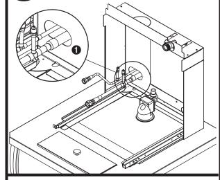
Braze supplied quick-connect lines onto stub-ins 1.
