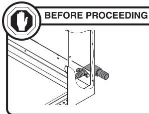
Prior to installing the docking assembly, ensure that the drain fitting is oriented (right or left) correctly for your installation. An optional straight drain fitting is also supplied. You may need to remove the back panel of the docking assembly in order to re-orient or change the drain fitting. Replace back panel prior to mounting the docking assembly.
