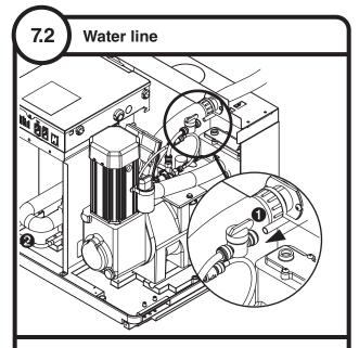
• Insert potable water line into valve 1
