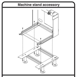
Mount docking assembly to machine stand accessory
