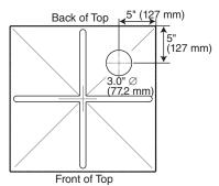
Locate hole position 5" (127 mm) from back and right of dispenser top
