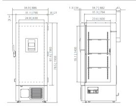
\*Note: External cabinet depth of 37.5" (952 mm) permits passage through a standard 38" (965 mm) doorway when rear stand-off brackets are removed, four screws. Bracket removal is not required for 40" (1016 mm) doorway.
