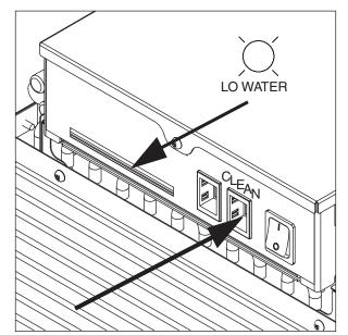
Mix 1 gallon (3.8 L) 120 F (49 C) water and 7 oz (198 g) (one 7 oz packet of Follett SafeCLEAN ice machine cleaner, P/N 00132001). Locate cleaning cup. Fill until HI WATER light comes on (Fig. 2).
