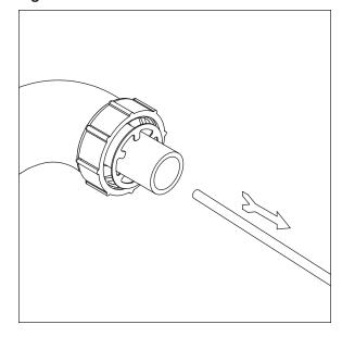
11. Reconnect coupling. Press power switch ON. Ice pushes Sani-Sponges through tube (Fig. 11).
