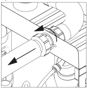
Using disposable food service grade gloves, insert dry Sani-Sponge TM (kit part# 00132068). Next,-insert Sani-Sponge soaked in Nu-Calgon IMS-II sanitizer solution. Push both Sani-Sponges down ice transport tube with supplied pusher tube
