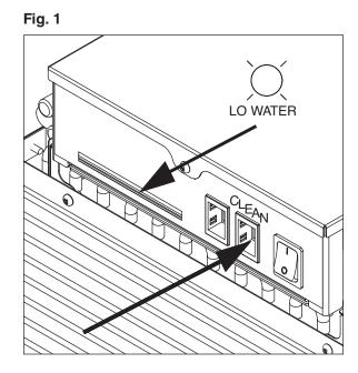
Mix 1 gallon (3.8L) 120°F (49°C) water and 7 ounces (198g) (one 7 ounce packet of Follett SafeCLEAN ice machine cleaner, part#-00132001). Locate cleaning cup. Fill until HI WATER light comes on (Fig. 2).
