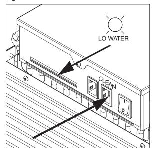
Mix 1 gallon (3.8L) 120°F (49°C) water and 7 ounces (198g) (one 7 ounce packet of Follett SafeCLEAN ice machine cleaner, part#-00132001). Locate cleaning cup. Fill until HI WATER light comes on (Fig. 2).
