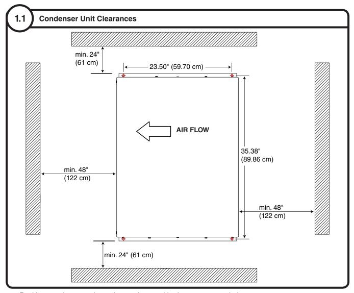
Position condenser unit as shown above, with clearances noted above
