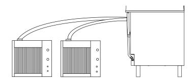
Automatic load units with two ice machines
