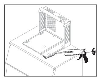
Seal perimeter of docking station to mounting surface.
