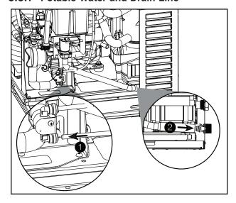
Insert potable water line into valve 1.
