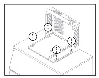
Mount louvered docking assembly using four screws provided.
