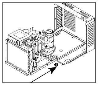
Slide ice machine into louvered docking assembly
