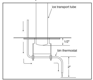
Lubricate transport tube with water then route transport tube and thermostat through grommet and into bin 1.
