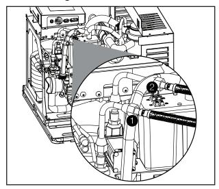
Connect cooling water supply 1 and return 2 lines (supplied and connected to inside of docking station) to ice machine (3/8" FPT).
