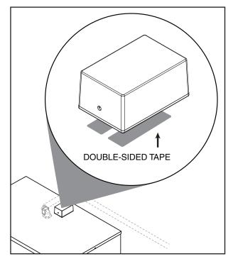
Apply double-sided tape to bottom of thermostat box and mount box on bin. 3.2 Install shuttle actuator and bracket
