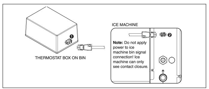
• Connect 2-pin bin thermostat cable at thermostat box on bin and at front of ice machine.
