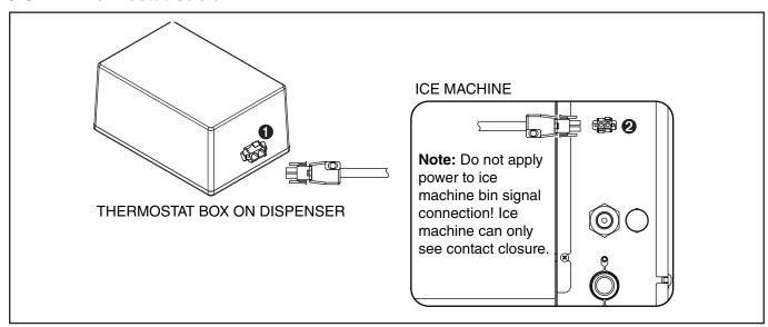
Connect 2-pin bin thermostat cable at thermostat box on dispenser and at front of ice machine.
