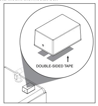
Apply double-sided tape to bottom of thermostat box and mount box on bin.
