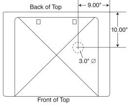
Locate hole position 10" (254 mm) from back and 9" (229 mm) from right of dispenser top.
