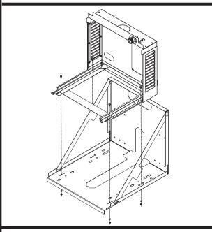
Mount louvered docking assembly to wall bracket accessory
