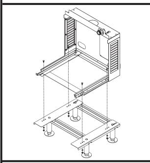
Mount louvered docking assembly to machine stand accessory
