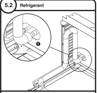
Braze supplied expandable refrigerant lines in place • Connect louvered docking assembly to ice machine.
