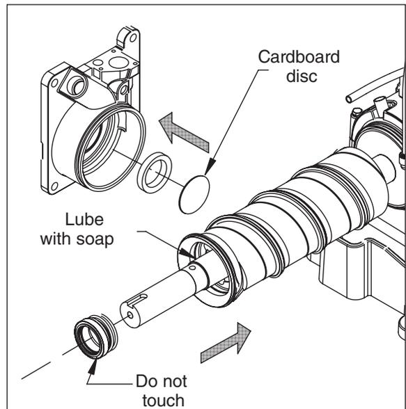
5. Reinstall main housing as shown.
