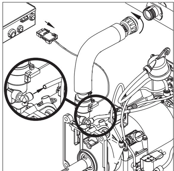
8. Loosen nut on V-band clamp and remove.
