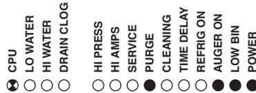
3. **Normal purge indicator.** After a selected period of ice making time has elapsed (1 or 2 hours), the ice machine will automatically self-flush. The compressor will shut down but the fan and gearmotor will continue to run. After the flush is complete the machine will refill and start without a time delay.
