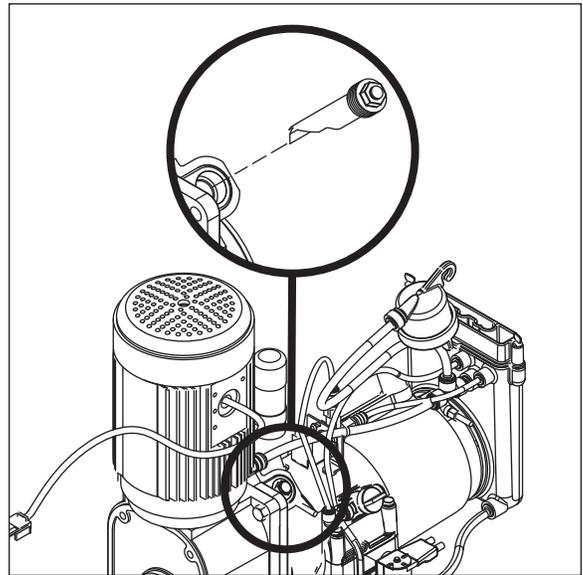
3. Unplug and remove gearmotor as shown.
