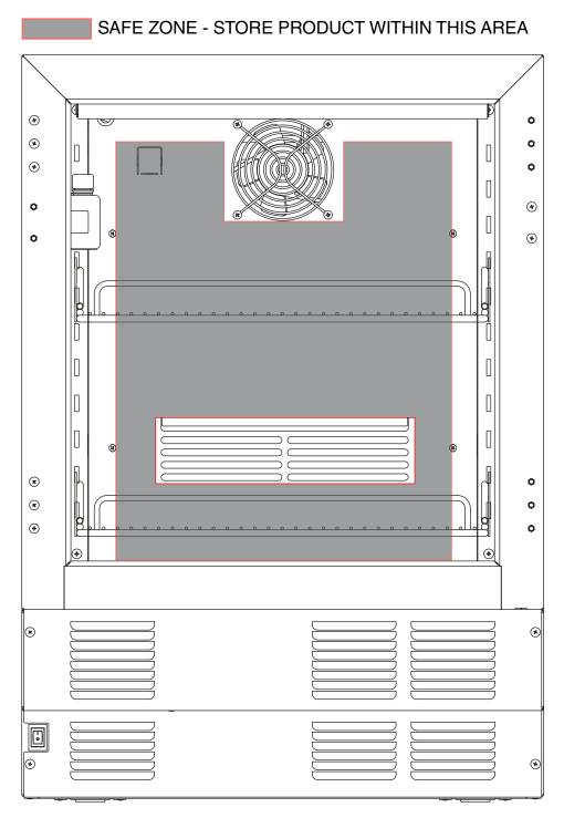
KEEP CLEAR 2" ON EACH SIDE AND TOP. FAN GRILL AND RETURN VENT MUST BE VISIBLE.
