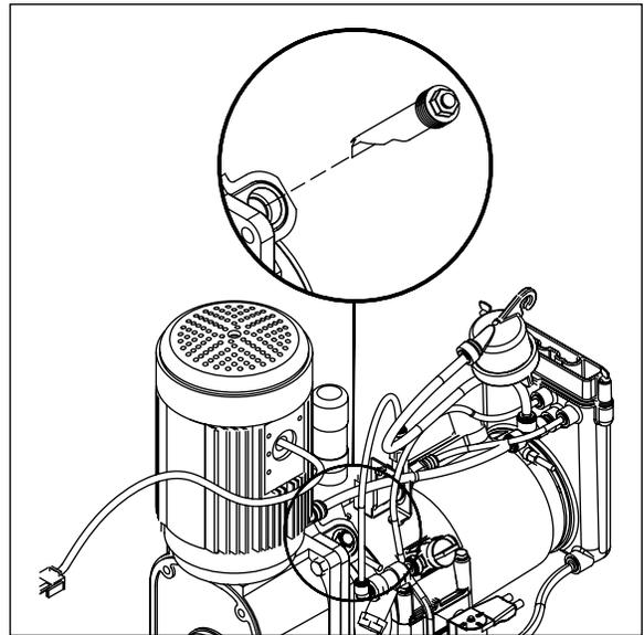
3. Unplug and remove gearmotor as shown.
