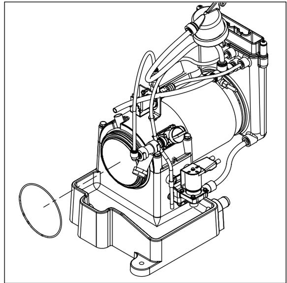
3. Press new mating ring into main housing as shown.
