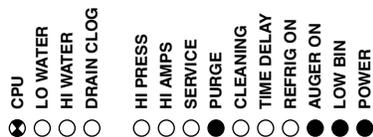
3. **Normal purge indicator.** After a selected period of ice making time has elapsed (2 or 6 hours), the ice machine will automatically self-flush. The compressor will shut down but the fan and gearmotor will continue to run. After the flush is complete the machine will refill and start without a time delay.
