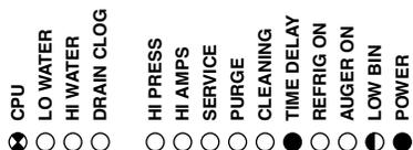
2. **Normal time delay.** When the bin fills with ice, the LOW BIN light goes out and the refrigeration and auger drive systems immediately shut down. (**Note:** The fan motor will continue to run for 10 minutes to cool condenser) The TIME DELAY light comes on, initiating the time delay period. When the time delay expires, the machine will restart provided that the LOW BIN light is on.
