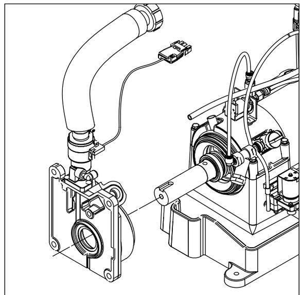
6. Orient auger shaft with keyway in the upward position.
