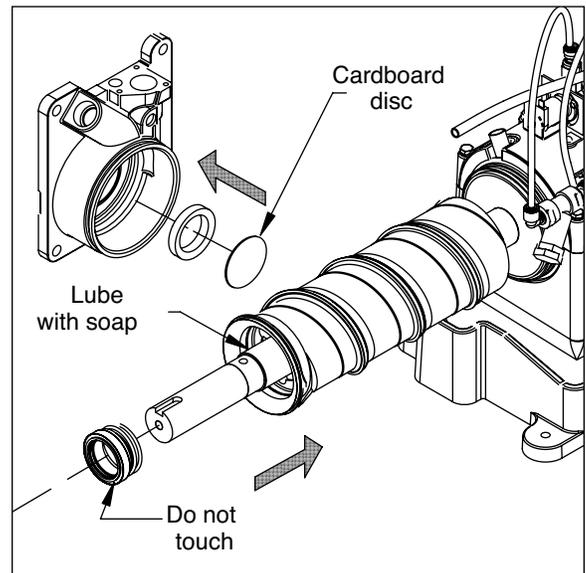
5. Reinstall main housing as shown.
