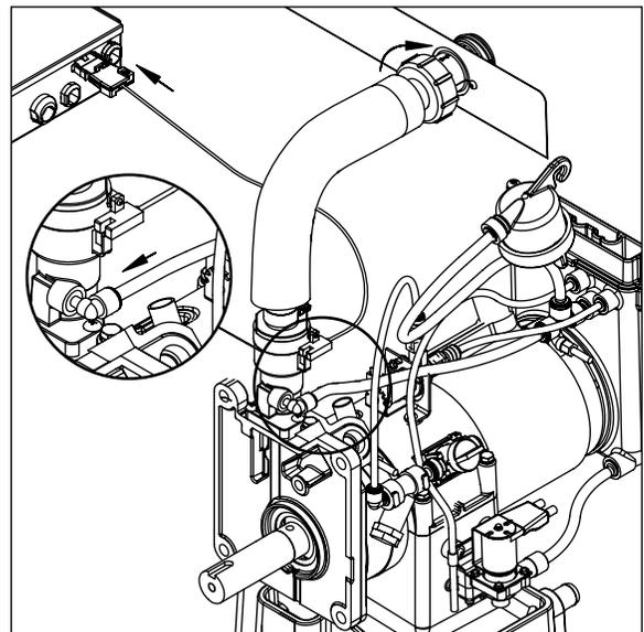
14. Apply a light coat of anti-seize compound to the auger shaft.
