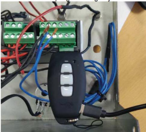
The programming key must be powered in order to be operational. Use a USB 5V/1A output to feed the key and a typeA USB/male Micro-B USB cable
