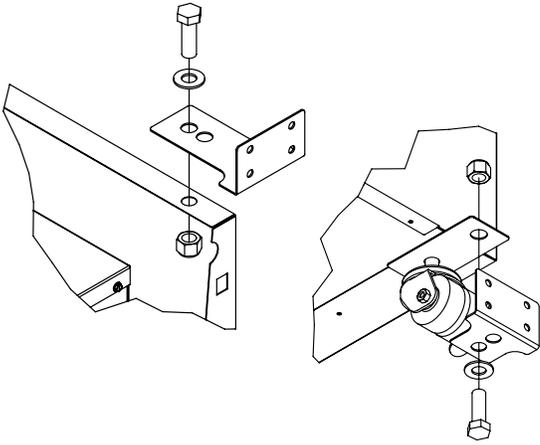
**Seismic anchoring kits for REF20i and REF25i refrigerators and all REF/FZR20/25/45 refrigerators and freezers**
