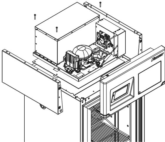
**Replacement CRS (complete refrigeration system) module for Infinity Series REF12i, REF20i and REF25i refrigerators**
