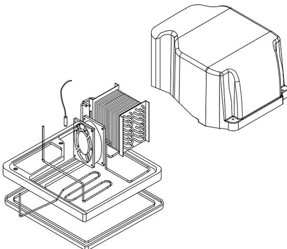
**Replacement CRS (complete refrigeration system) module for REF12-LB refrigerators**
