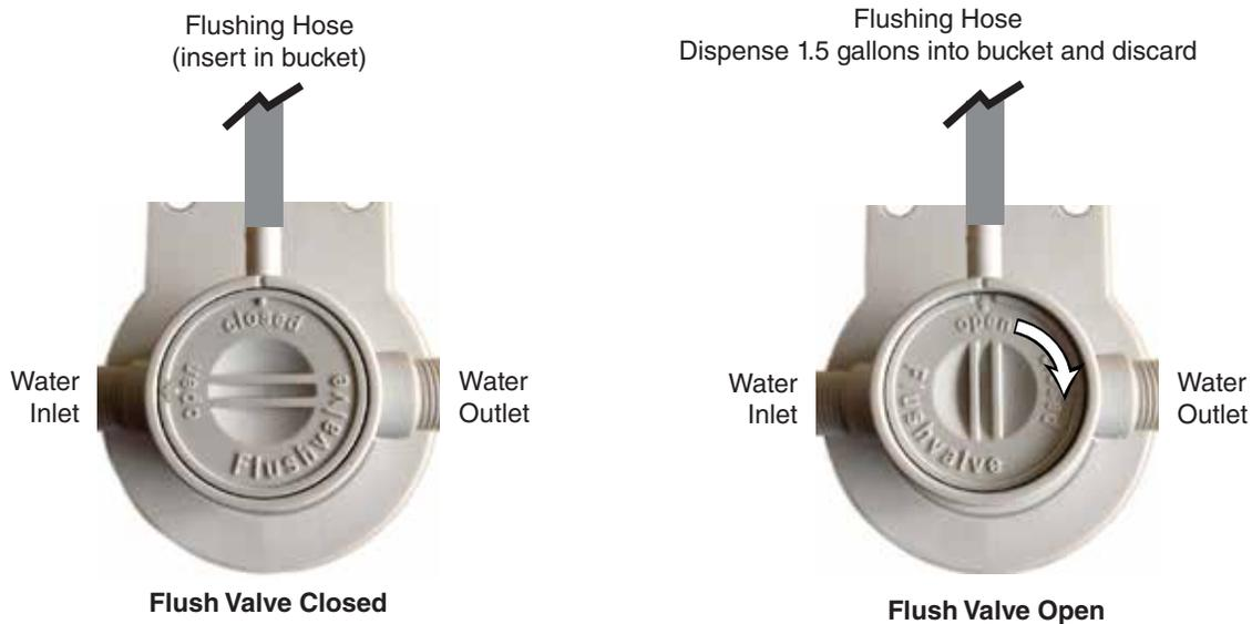
5. Rotate the flushing valve to "CLOSED" (with "OPEN" pointed to exit port of manifold).
