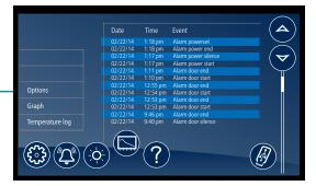
Temperature log – access a chronological listing of logged temperatures, starting with the most recent
