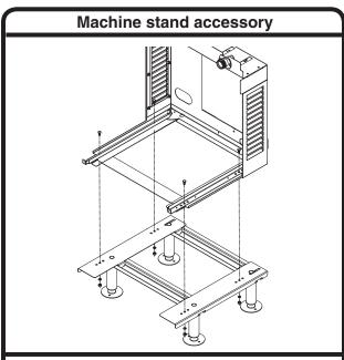
Mount louvered docking assembly to machine stand accessory
