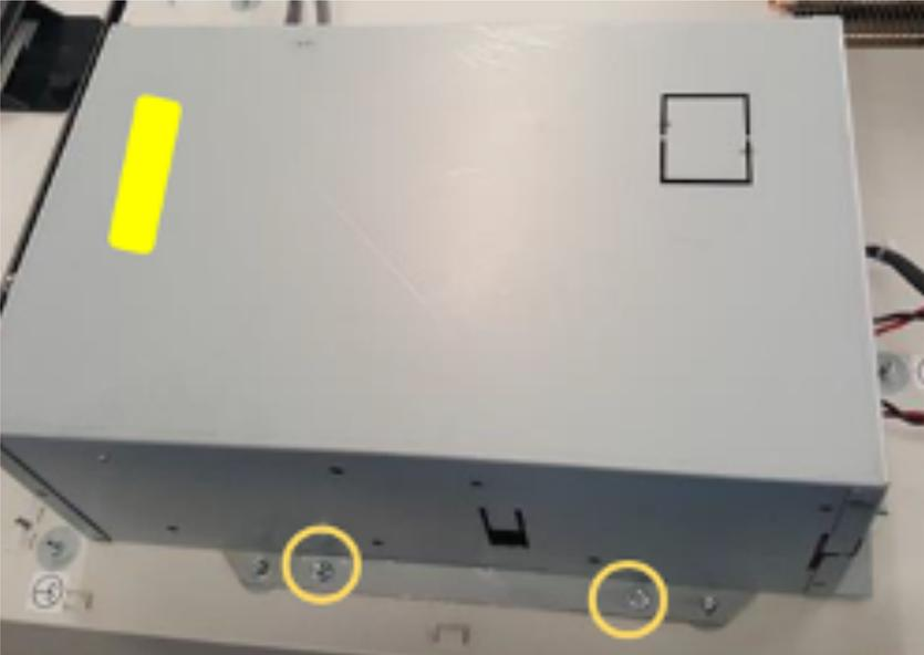
4. Lift the cover to gain access to the electrical connection between the enclosed electronics in the cover and the power supply.
