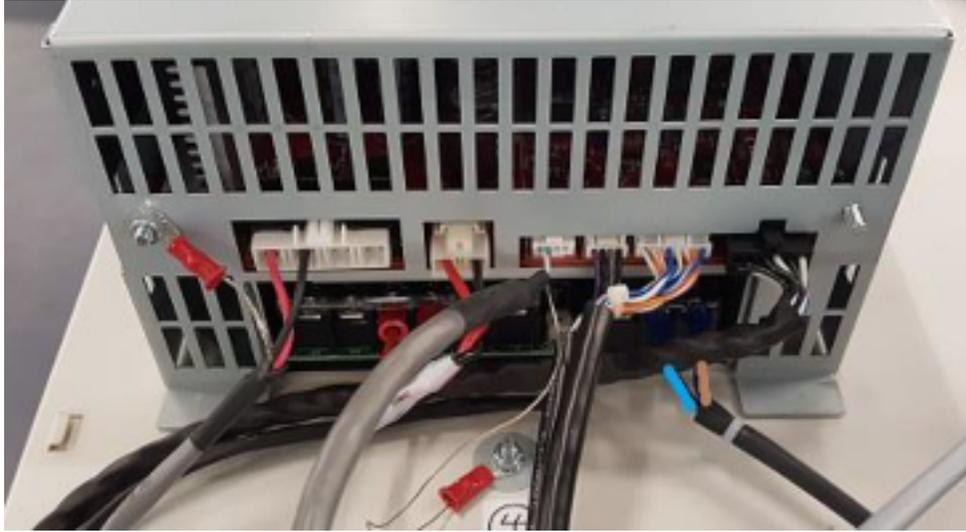
13. Secure the cables running beside the power supply cover with a zip tie placed around the cables and through the zip tie anchors located on the side of the power supply cover.
