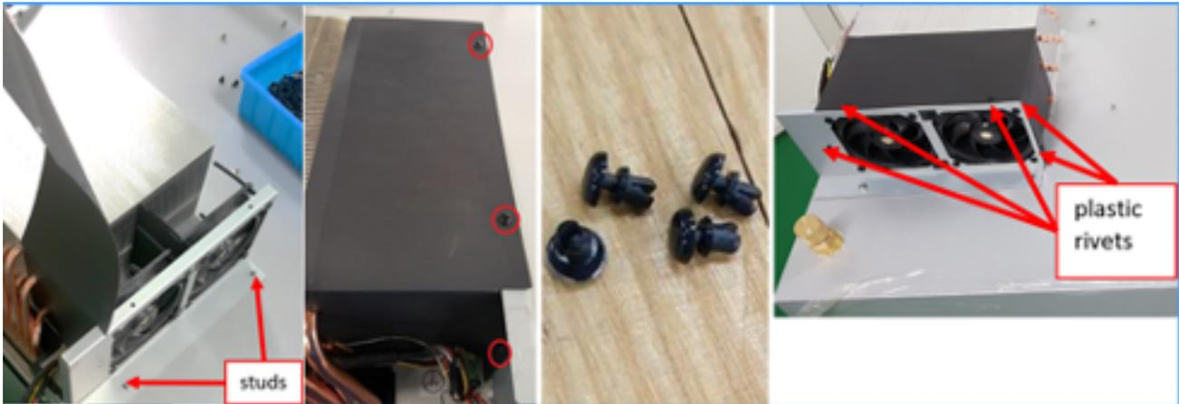
8. Reinstall the top cover (Refer to the section Removing the Top Cover).
