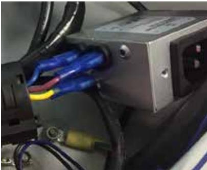
2. Align the receptacle with the cutout in the painted steel and secure with the Phillips head screws and washers.
