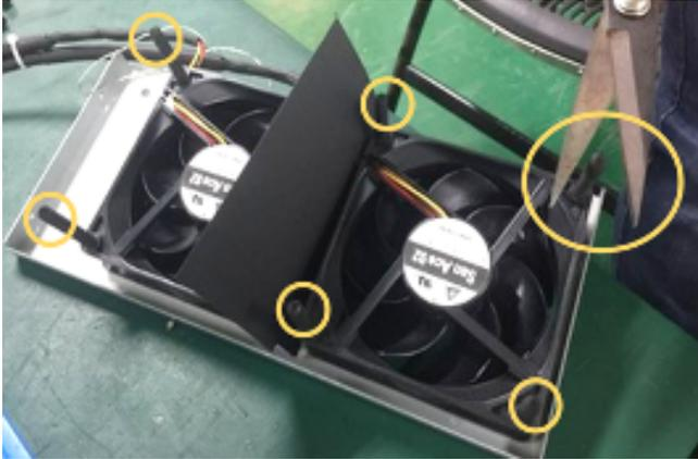
Note: Make sure the fans are installed with the fan label facing the heat exchanger.
