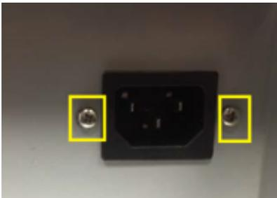
3. Pull the power receptacle towards the power supply, freeing the receptacle from the painted steel.
