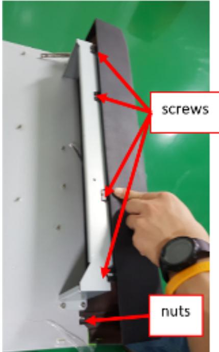
3. Remove the two outside nuts (one on each side of the panel).
