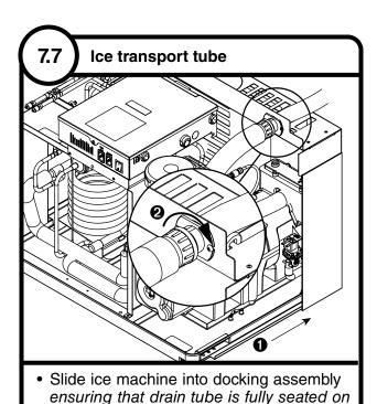
Insert ice transport tube into coupling and
