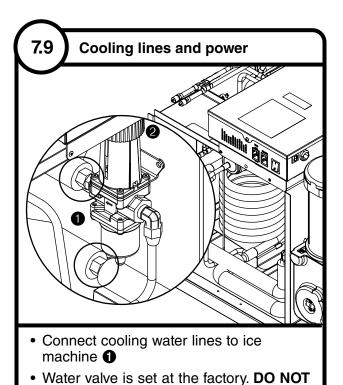
remove seal or adjust water valve 2
