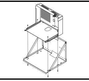
Mount docking assembly to wall bracket accessory
