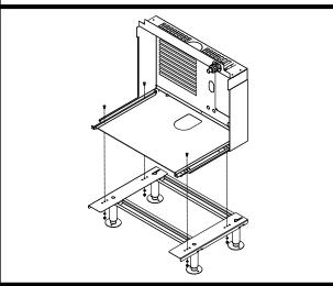
Mount docking assembly to machine stand accessory
