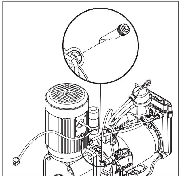
3. Unplug and remove gearmotor as shown.
