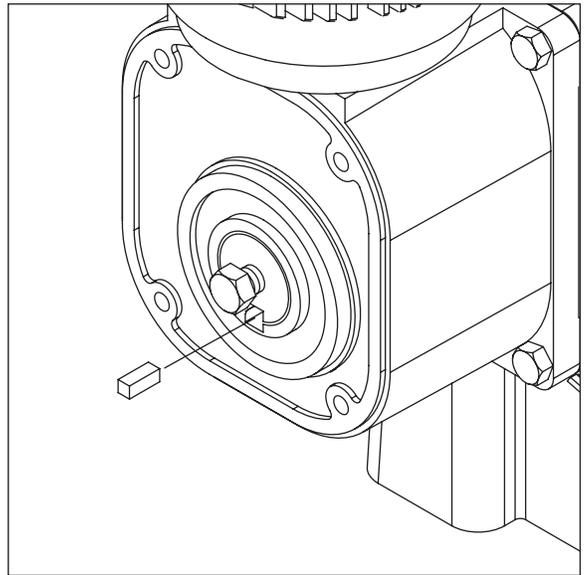
20. Remove bolt and reinstall the washer and bolt. Place retainer over bolt and secure with nut and washer.
