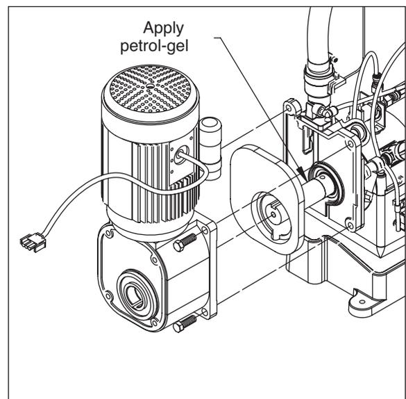
18. Using a wrench, rotate the shaft clockwise to align the keyways in the gear housing and the shaft so as to accept the key.
