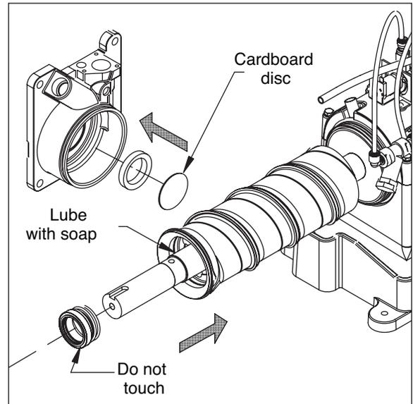
5. Reinstall main housing as shown.
