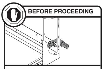
Prior to installing the docking assembly, ensure that the drain fitting is oriented (right or left) correctly for your installation. An optional straight drain fitting is also supplied. You may need to remove the back panel of the docking assembly in order to re-orient or change the drain fitting. Replace back panel prior to mounting the docking assembly.
