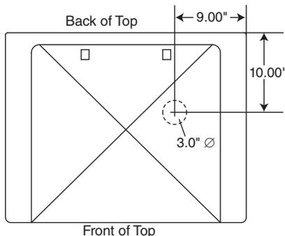
Locate hole position 10" (254 mm) from back and 9" (229 mm) from right of dispenser top
