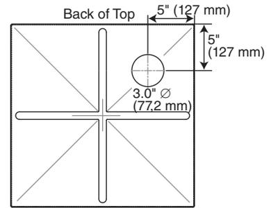
Locate hole position 5" (127 mm) from back and right of dispenser top
