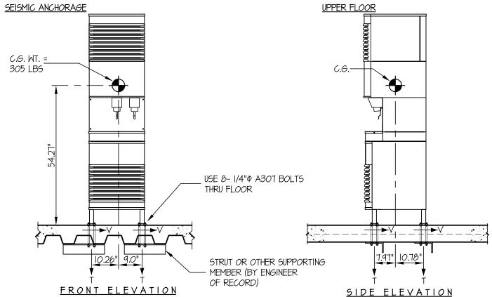
LOADS: PER 2001 CALIFORNIA BUILDING CODE - SECTION 1632A (WORKING LOADS, NOT ULTIMATE)
