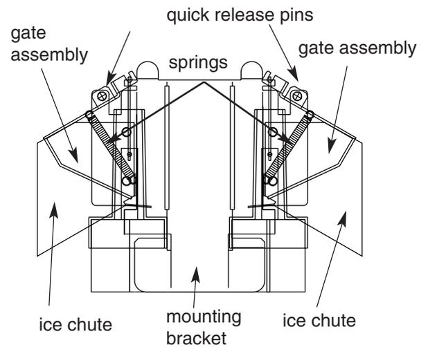
U300 cutaway – front view
