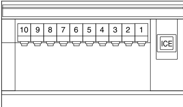
**Valve position #1 is always next to ice tower. Right-hand unit shown.**
