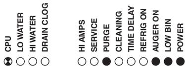
3. **Normal purge indicator.** After a selected period of ice making time has elapsed (1 or 2 hours), the ice machine will automatically self-flush. The refrigeration system will shut down but the gear motor will continue to run. After the flush is complete the machine will refill and start without a time delay.
