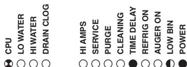
2. **Normal time delay.** When the bin fills with ice, the LOW BIN light goes out and the refrigeration and auger drive systems immediately shut down. The TIME DELAY light comes on, initiating the time delay period. When the time delay expires, the machine will restart provided that the LOW BIN light is on.
