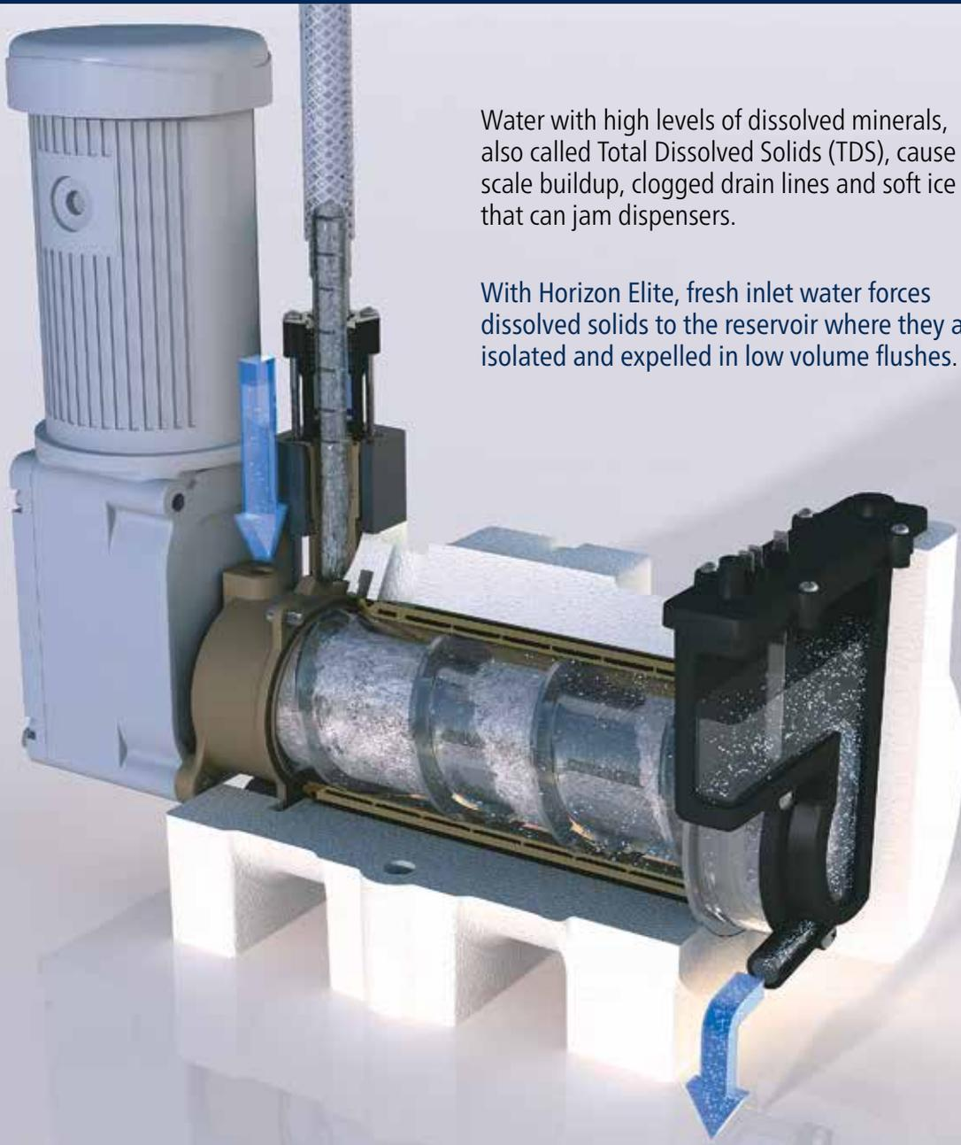
Water with high levels of dissolved minerals, also called Total Dissolved Solids (TDS), cause scale buildup, clogged drain lines and soft ice that can jam dispensers.
